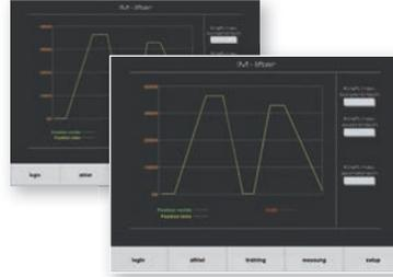
Apart from logging training data, the device also has the capability to perform force measurement in a lifting and lowering direction. The measurements can be carried out isometrically with freely selectable positions as well as isokinetically with freely selectable rates of velocity and acceleration.
