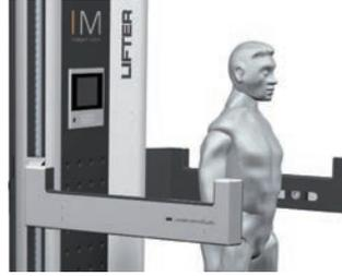
A maximum and minimum movement threshold can be set in order to limit the overall movement space of the device. The body scan function simplifies the setting of these limits. The arms of the device and barbell are moved into the desired position, then a button is pressed to set this position as limit and save the setting.
