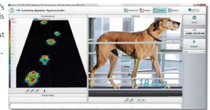
The system consists of a treadmill equipped with a calibrated pressure sensor matrix and one or several synchronised cameras.
